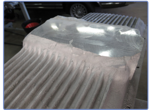
Figure 3 - Cold sprayed oil pan prior to machining.
