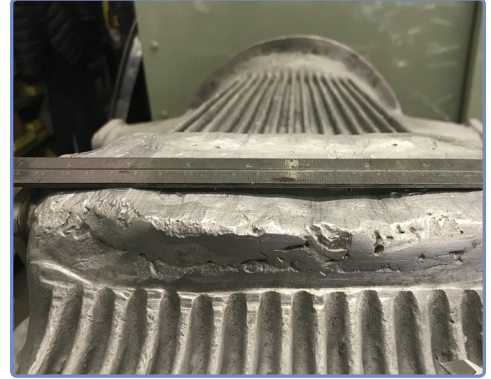
Figure 2 - Leaks caused by visible cracks and unacceptable aesthetics inside and outside the oil pan.
