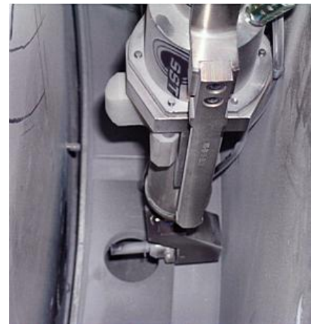
Cold Spray Gun Inside the Reactor Annulus
