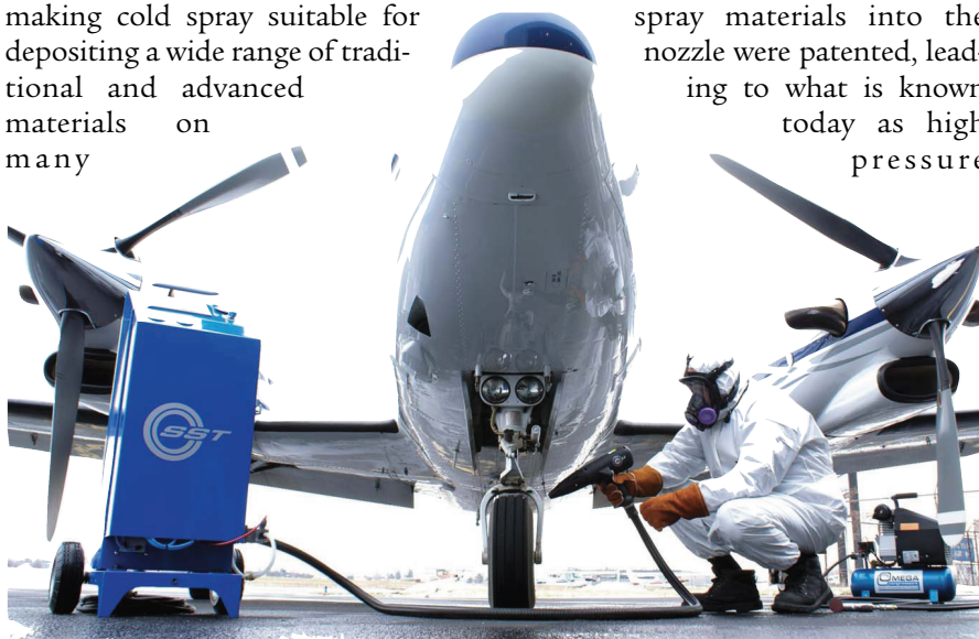
Figure 1: Field repair of corrosion surface damage by low-pressure cold spray.
