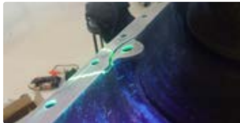
Figure 2. (b) Liquid penetrant inspection of the cover
