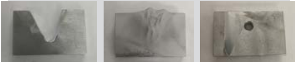
Figure 4. Simulation coupons (a) before spraying; (b) as sprayed; (c) machined to tolerance
