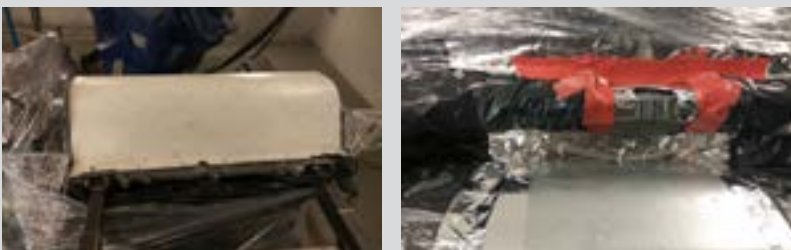
Figure 5. Engine lower crank case masked prior to cold spray operation
