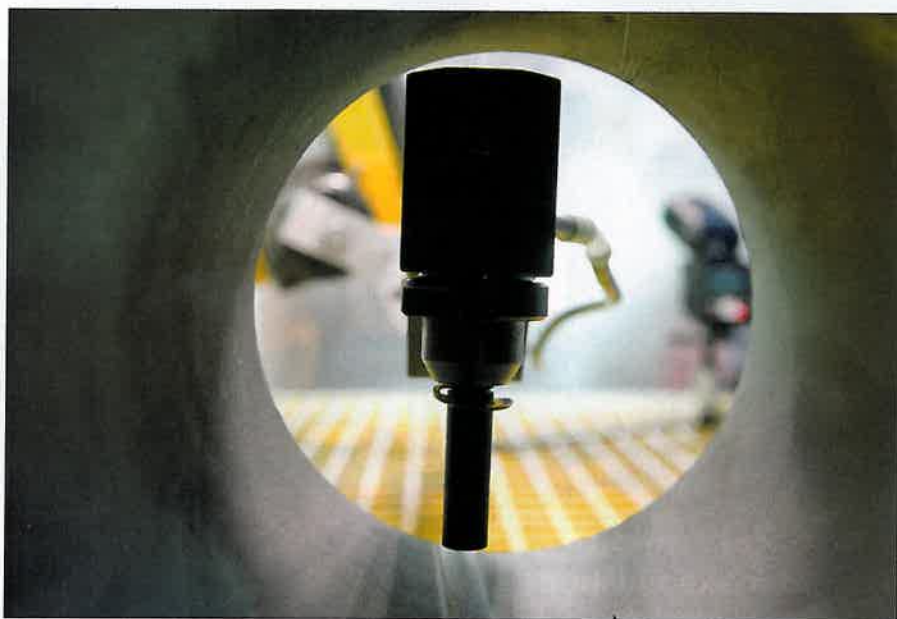
Low-temperature deposition of the inside of an aluminum tube using low-pressure cold spray. (Photo courtesy of CenterLine Windsor Ltd.)
