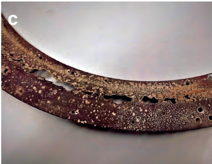
Fig. 1 — A — Rear gun turret (Photo by Paulspixs/DepositPhotos); B, C — part of a heavily corroded turret mounting assembly showing through-thickness corrosion holes. (Photos B and C are courtesy of CenterLine Windsor Ltd.)
