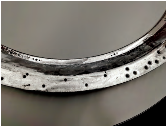
Fig. 3 — The component cold sprayed and grinded. (Photo courtesy of CenterLine Windsor Ltd.)
