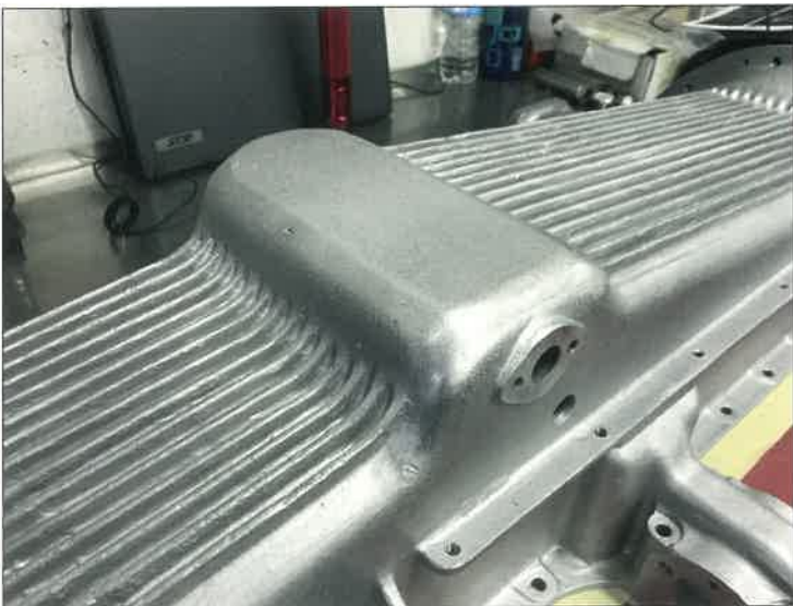
Fig. 3 — Restored oil pan. (Courtesy of RX Autoworks.)
