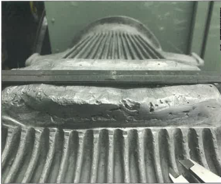
Fig. 1 — Visible cracks and unacceptable aesthetics are seen around the oil pan.
