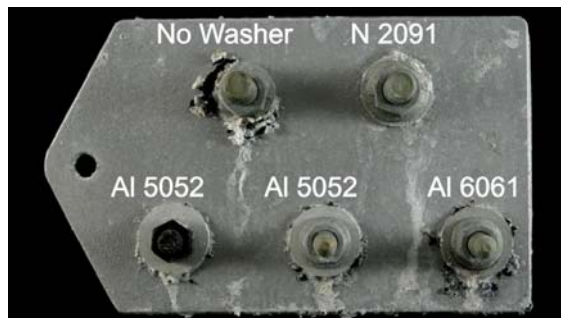
Fig. 5. Conversion-treated and powder-coated magnesium AM60 alloy plate after 40 days testing following the GM9540P standard. This sample shows different levels of corrosion when utilizing aluminum washers of various compositions coupled with different nuts. Note that, even in powder-coated magnesium, severe galvanic corrosion may still occur if no aluminum washer is utilized [7].
