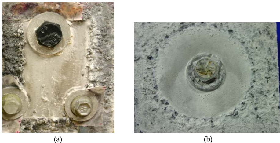
Fig. 13. (a) Magnesium casting alloy AE44 plate on which the central area was selectively cold sprayed with aluminum, after 100 hours of salt-spray exposure, as per ASTM B117. Note that the cold-sprayed area (between the three washers) is free of corrosion attack. (Courtesy of CANMET-MTL, Natural Resources Canada) (b) Magnesium alloy AM60 plate, where the area surrounding the fastener hole was selectively cold sprayed with aluminum, after 1000 hours corrosion test, as per ASTM B117. (Courtesy of NRC Integrated Manufacturing Technologies Institute , London, Ontario, Canada)
