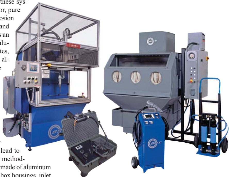
Fig. 3 — Various stand-alone configurations of low-pressure cold-spray equipment including auxiliary components. Courtesy of CenterLine Windsor Ltd.
